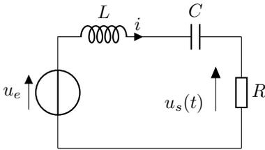
1.1  $\frac{u_s}{u_e} = \frac{R}{R + j\omega L + Z_c} = \frac{jRC\omega}{1 + jRC\omega - LC\omega^2}$
